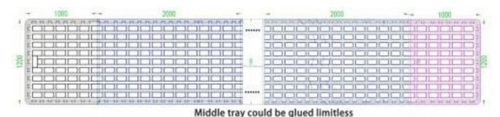
**Infinity Trays** are designed to easily connect multiple trays together, end-to-end. Each tray ends with connection point, connection point end overlap on the normal ends for a snug fit when connecting trays. Use an suitable adhesive on connection point end, then attach the normal end overlap firmly on top of it. This allows for a level growing surface across multiple tray pieces.
